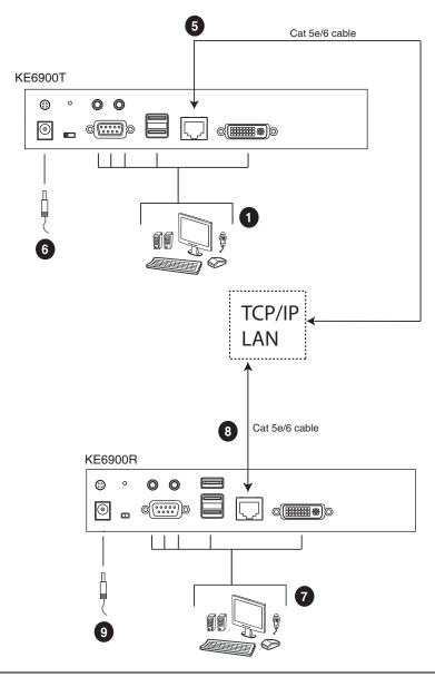
**Note:** The diagram above shows the KE6900T and KE6900R. The KE6940 installation is the same except that an additional DVI monitor can be connected at each end for a dual-view display setup.
