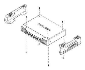
2. Remove four screws from the units and then use the same screws to secure the units together with the link bracket provided with the kit.
