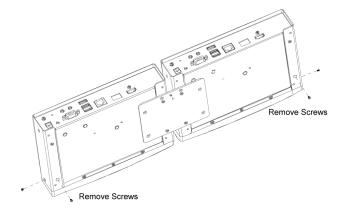
4. Use the screws in step 3 to install the left and right mounting brackets.
