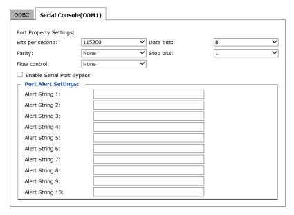
Select the values that match the ones used by the connected serial console device. The port property settings that the CN9600 supports are as follows:
