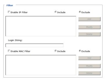
To enable IP and/or MAC filtering, check IP Filter Enable and/or MAC Filter Enable.
