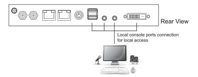
This access is like you using the server/computer directly. The CN9600 is able to split the signal to both the local and remote consoles.
