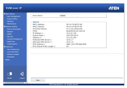
The Main screen consists of the user menu in the left panel, with a *Viewer* icon (to launch the Java or WinClient Viewer) as well as a *Logout* icon displayed in the bottom of the menu.
