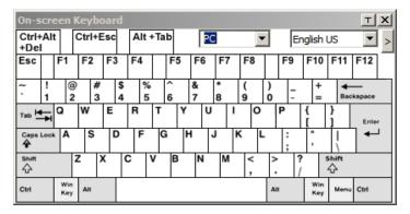
One of the major advantages of the on-screen keyboard is that if the keyboard languages of the remote and local systems are not the same, you do not have to change the configuration settings for either system. The user just has to bring up the on-screen keyboard; select the language used by the computer on the port he is accessing; and use the on-screen keyboard to communicate with it.
