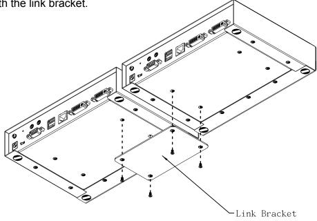
2. Remove the bottom and side screw from each KE6900 unit.
