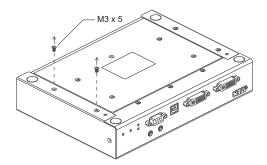
2. Use the screws from step 1 to screw the mounting bracket to the bottom of the Transmitter as shown below:
