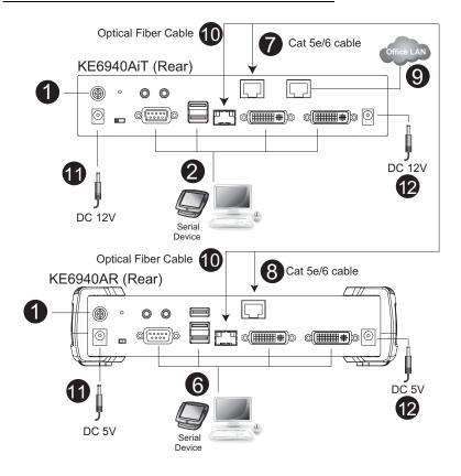
**Note:** The diagram above shows the KE6940AiT setup with a KE6940AR. The KE6900AiT installation is the same except with one less DVI monitor setup.
