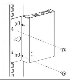
**Note:** Rack screws are not provided. We recommend that you use M5 x 12 Phillips Type I cross recessed type screws.
