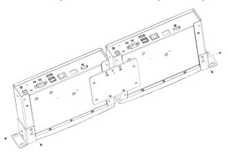
5. Screw the mounting brackets to the rack.
