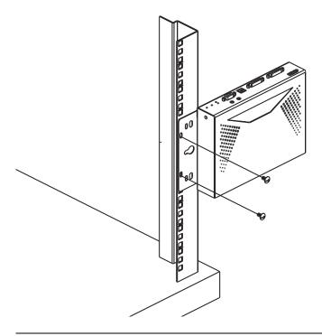
**Note:** Rack screws are not provided. We recommend that you use M5 x 12 Phillips Type I cross recessed type screws.
