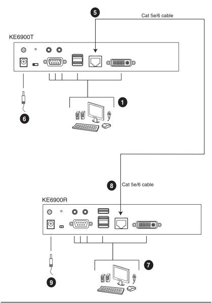
**Note:** The diagram above shows the KE6900T and KE6900R. The KE6940 installation is the same except that an additional DVI monitor can be connected at each end for a dual-view display setup.
