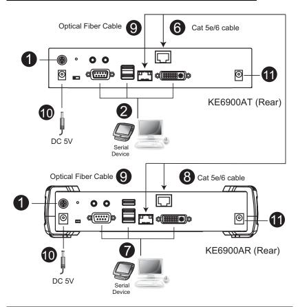
**Note:** The diagram above shows the KE6900AT and KE6900AR. The KE6940A installation is the same except that an additional DVI monitor can be connected at each end for a dual-view display setup.
